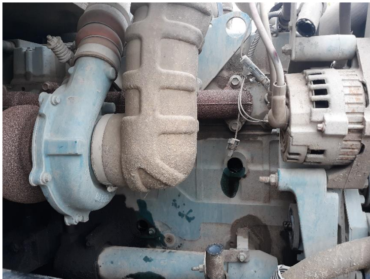
Figure 8. Holes drilled in 1996 International 4700 engine block.
